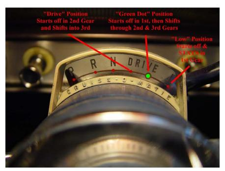
The illustration above shows the functions of each of the forward gear positions of the shifter. The function of each of the shifter positions are as follows:
