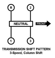
The illustration above shows the shift pattern for the 3-speed manual transmission with column shifter:
