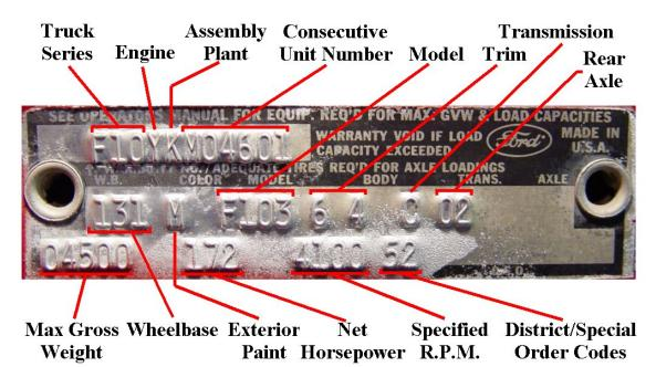
The codes used on this particular vehicle decode as follows:
